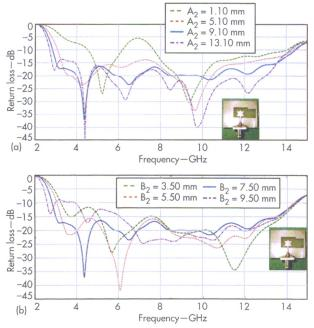
3. These plots show the effects of antenna parameters (a)  ${\rm A}_2$  and (b)  ${\rm B}_2$  on return loss.
