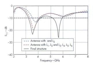
These curves show the simulated VSWR performance for the three antennas in the antenna design process.
