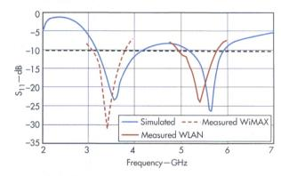
4. The curves plot the simulated and measured  $S_{11}$  behavior of the proposed antenna.
