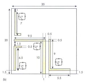
1. The configuration in (a) shows top view of the antenna structure and (b) shows bottom view of the antenna structure.
