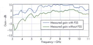
9. These plots show the peak gain for the prototype antenna with and without FSS across a frequency range of 3 to 11 GHz. The gain increased by about 4 to 5 dBi with application of the FSS .
