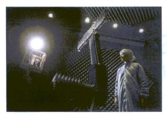
2. The Spherical Near-Field Antenna Test Facility (SNFTF) can test an antenna's behavior in the near-field and extrapolate far-field behavior using this data. (Courtesy of European Space Agency)
