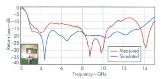
The plots show the measured and simulated reflection coefficients for the UWB antenna.
