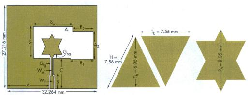
1. These diagrams show the geometry of the star-shaped UWB antenna.
