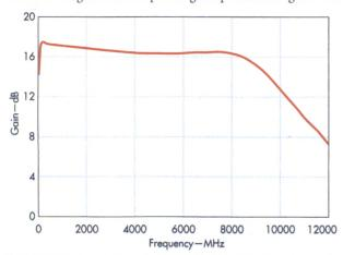
Model GVA-123+ is a broadband amplifier in an SOT-89 package with gain within ±0.7 dB through 8 GHz.
