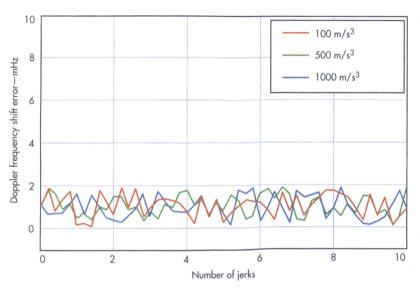
5. This plot shows simulation errors of Doppler frequency shifts with different jerk rates applied.
