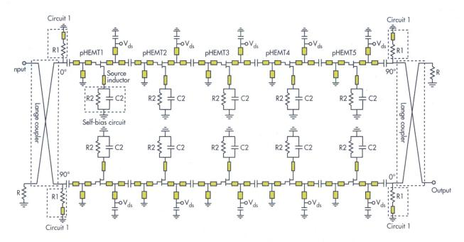
2. This circuit topology shows the pHEMT MMIC LNA and its use of multiple pHEMT devices and Lange couplers at the input and output ports to achieve high gain and low noise figure at Ka-band frequencies.
