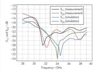
6. These plots show the  $S_{11}$  and  $S_{22}$  performance of the LNA with  $V_{ds}$  and  $V_{qs}$  of +2 VDC and -0.19 VDC, respectively.
