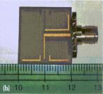
3. These are (a) top and (b) bottom views of the fabricated antenna.
