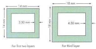
These are the unit-cell dimensions for the three layers of antenna FSS.
