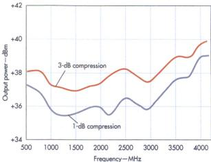
The upper trace shows output power at 1-dB compression and the lower trace is output power at 3-dB compression for the model ZHL-5W-422+ amplifier.
