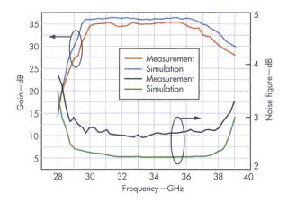
5. These plots show the simulated and measured noise figures and associated gains for the LNA with drain-source voltage ( $V_{\rm gs}$ ) and gate-source voltage ( $V_{\rm gs}$ ) of +2 VDC and -0.19 VDC, respectively.
