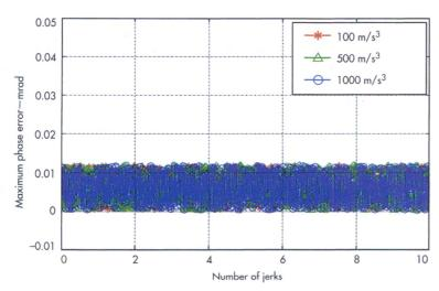
3. These are simulation results for maximum phase errors with different amounts of jerk applied.
