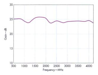
The small-signal gain of the model ZHL-5W-422+ amplifier remains flat through 4.5 GHz.
