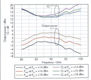
These curves show the quadrupler's simulated output power and conversion loss (CL).
