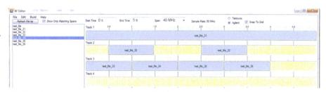
RF Editor boasts 10 independent tracks into which waveforms or waveform sequences can be moved and then reconnected to form a single file.
