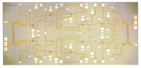
This microphotograph reveals the amplifier fabricated with the commercial pHEMT process.
