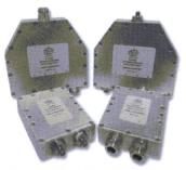
**Low Frequency Power Combiners** MECA introduces Low Frequency addition to the H-Series, 100-watt Wilkinson high power combiner/dividers. Available in 2 & 4-way configurations covering 5 to 500 MHz. VSWR of 1.30:1 accommodating load VSWR's of 2.0:1
