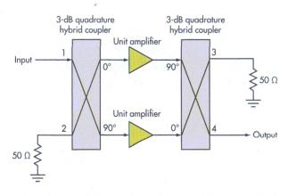
This circuit schematic diagram represents the balanced millimeterwave amplifier, which features two identical unit amplifiers and two quadrature hybrid couplers.
