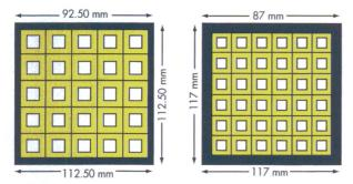
5. These are the overall screen dimensions for the different FSS layers.
