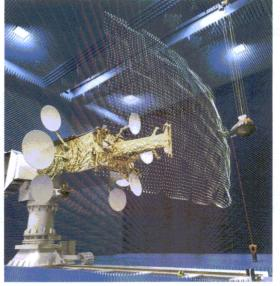
1. The Portable Antenna Measurement System (PAMS) can perform near-field probing along a planar or tilted surface using laser trackers for precision measurements. (Courtesy of Astrium GmbH)
