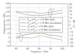
These curves compare the measured and simulated performance with frequency for the quadrupler.
